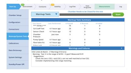
The Warmup Tests take less than 15 minutes. If the tests reveal any issues, resolve them before taking measurements.
