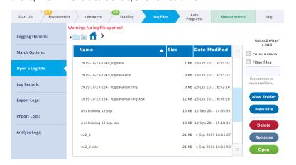
You can configure automatic matching under Log Files > Match Options. Or match manually under the **Measurements** tab.
