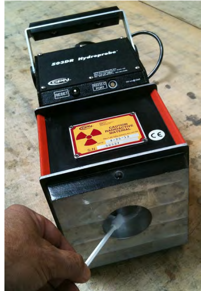
Figure 3.1 Leak Test Procedure
